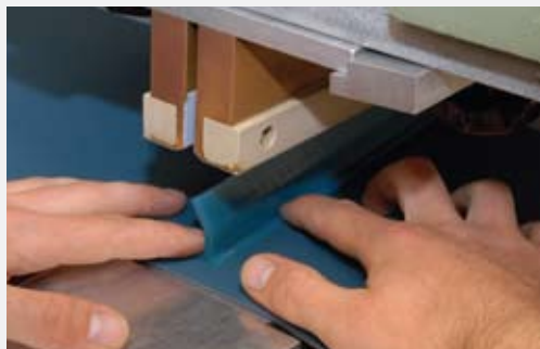
Figure right hand side: Automatic weld- ing of side walls
