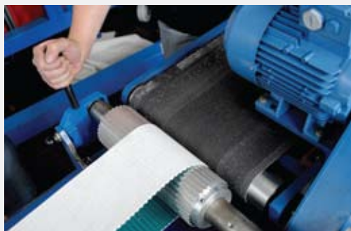
Surface grinding and finishing for belts up to 300 mm are available – for conveyor belts as well as timing belts.
